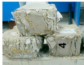
Figure 7: Collapse form of M(4/25)
