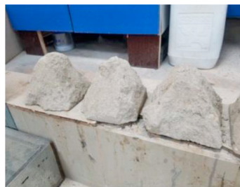
Figure 6: Collapse form of M(0)
